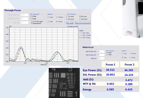
Designed to offer lens manufacturers real-time, high quality measurements of the optical power and modulation transfer function (MTF), the PMTF measures and characterizes every type of IOL (refractive & diffractive).
